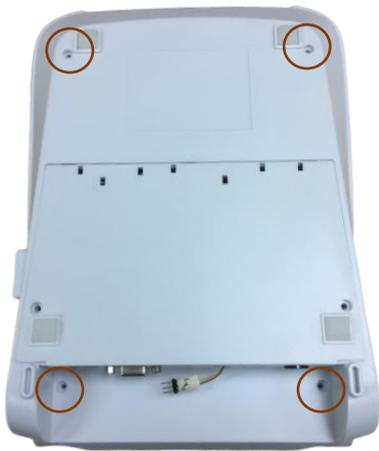
4. Turn the printer upside down, remove the four screws located on the bottom cover, and open the bottom cover
