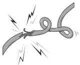
Do not bend the wire and do not allow the wire to be pressed by heavy object.
