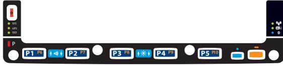
The integrated keypad contains five programmable keys, a blue modifier key and an orange modifier key.
