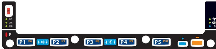
There are five integrated programmable keys located on the Thor VM2 below the display. Each programmable key can be modified by the Orange key for a total of 10 programmable keys.
